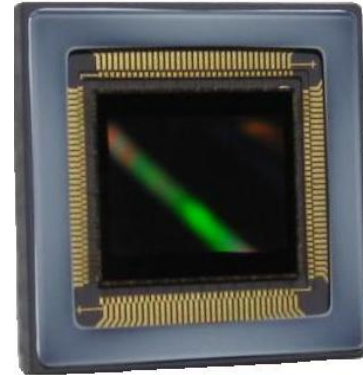
Fig.1. The photograph of a Color AM41V4 CMOS Image Sensor
